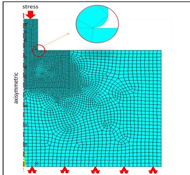
Figure 1: Construction of elements in impression creep test
