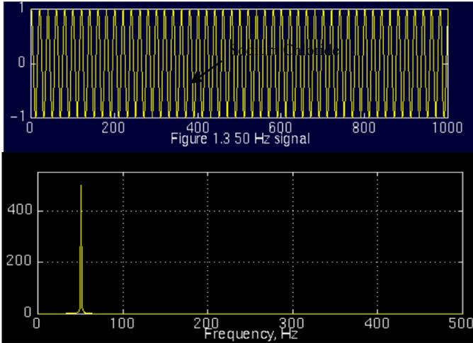
Fig. 1. up) AC power signal; down) furrier transform of AC power signal [12].
