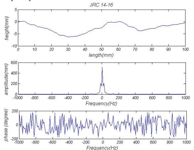
Fig. 3. a) Profile of JRC 14-16 b) amplitude vs. frequency diagram for FFT analysis of JRC 14-16 c) phase vs. frequency diagram for FFT analysis of JRC 14-16.
