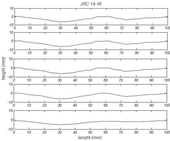
Fig. 4. The first diagram is 14-16 JRC profile and the others up to down are low pass filtered profiles with cutoff frequencies 990, 495, 100 and 20 Hz.
