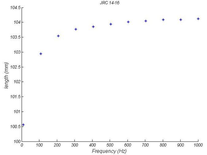
Fig. 6. Variation of actual length of profile vs. cutoff frequency of low pass filter for 14-16 JRC profile.
