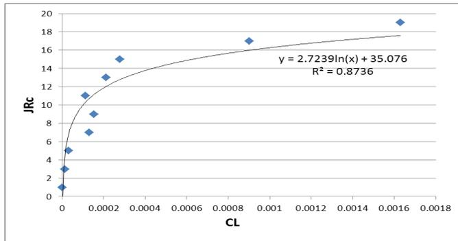
Fig. 7. Relation between JRC and  $CL$  for JRC profiles.
