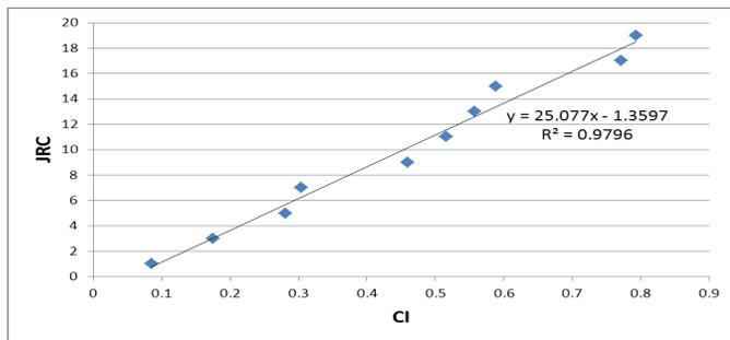
Fig. 10. Relation between JRC and CI for JRC profiles.
