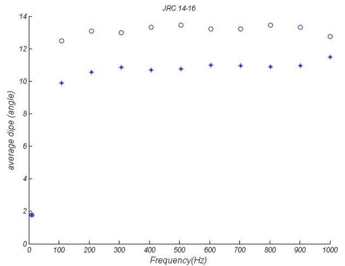
Fig. 8. Variation of average dip angle of profile vs. frequency of low pass filter for two different directions of 14-16 JRC profile (star: left to right; circle: right to left).
