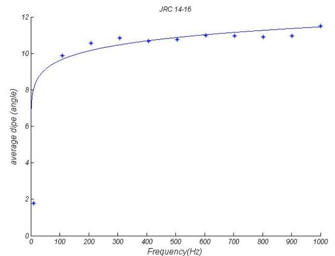
Fig. 9. The exponential equation that is fitted on variation average dip angles for 14-16 JRC profile (left to right).
